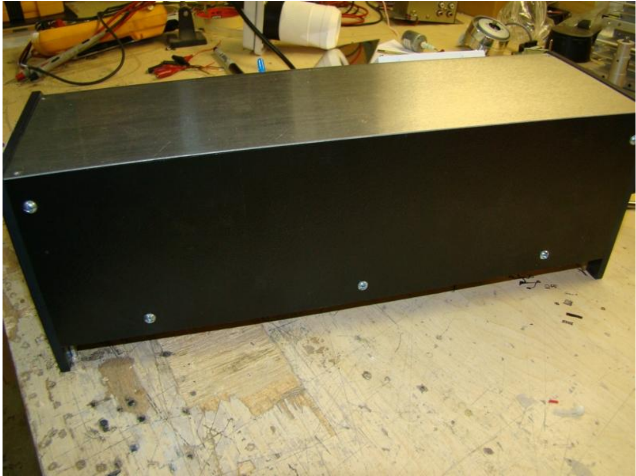
The Back, again 0.25" ABS. I left a 1" gap at the bottom for air flow.
